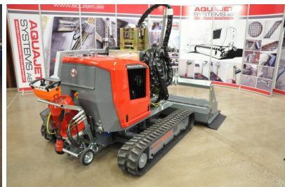
Hybrid drive-unit connected to the AQUA CUTTER
